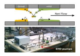
TA14- Michal Talmor, Worcester Polytechnic Institute: Developed predictive electrohydrodynamic models and discovered that differences in pressure generation between different conduction pumps were a function of the working fluid temperature. This was a new finding and, with her new model, led to the conclusion that small (micro-scale) EHD conduction pumps increase performance in low temperature areas, whereas larger pumps increase performance in high temperature areas.
